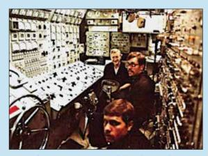
Fig. 11. The Maneuvering Room while underway. The area is rather narrow, with additional panels and gauges behind the watchstanders.
