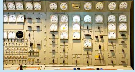
Fig. 10. The right-most panel controls the SSTGs and electrical distribution to the different busses which distribute electrical power. Both AC and DC current are provided. In older submarines, a motor/generator set was employed for AC/DC and DC/AC conversions; newer submarines use solid-state rectifiers.
