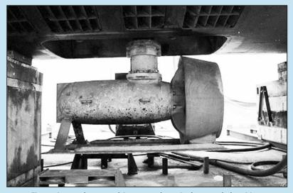
Fig. 17. A secondary propulsion motor shown in the extended position.
