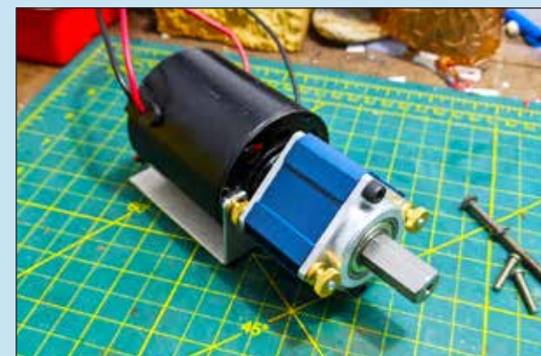
Fig. 15: Motor and gear box; initial test fit.
