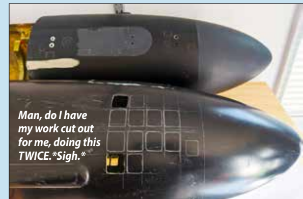
Fig. 12: The SSY bow, with scribing and VLS Tubes #15 & #16 open.
