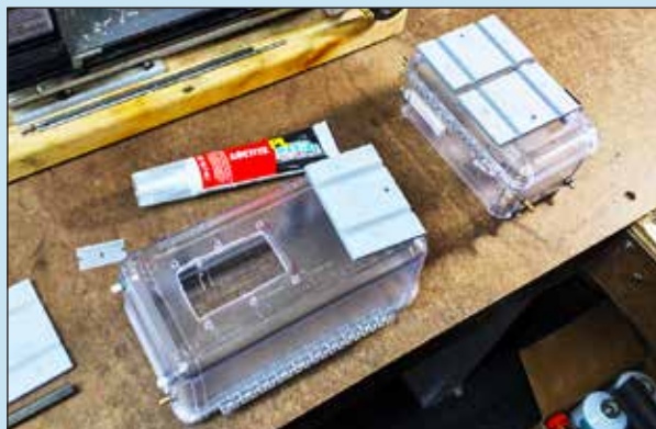
Fig. 19: Thermal cutout; 3-D printed PLA+ mounting plates.
