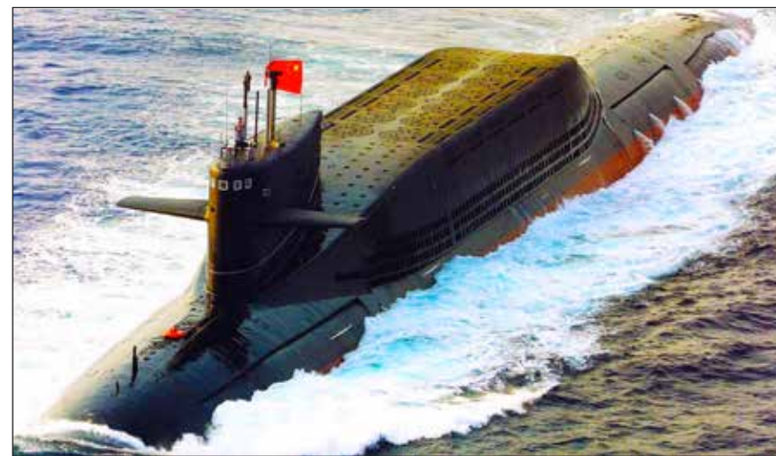
Fig. 22. Topside view of the Type 094 Jin class, with its twelve missile tube hatches visible.
