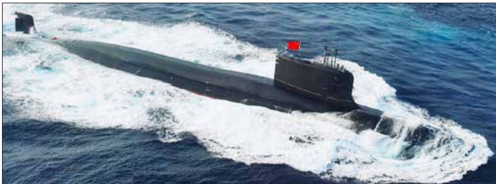
Fig. 18. The improved Type 093A (or G - "Gai") SSN with a noticeable fillet at the leading edge of the sail and a "hump" abaft it for a towed array reel, deployed from the upper rudder.
