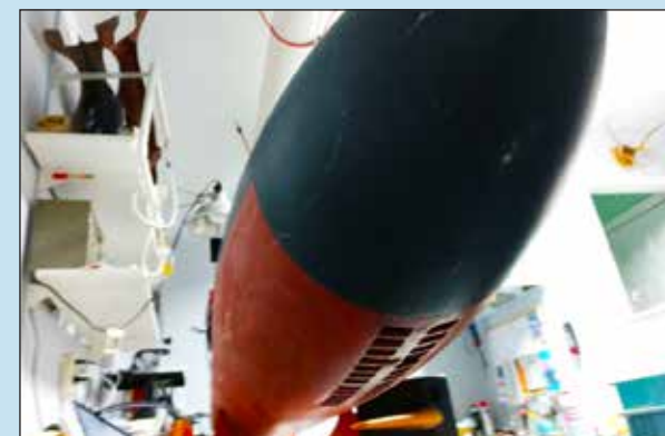
Fig. 6: Ventral view of the bow; note ballast flood holes in keel.
