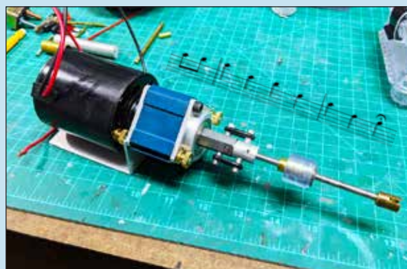
Fig. 17: The complete motor/gear box output shaft drive.
