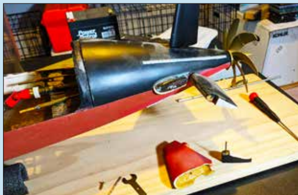
Fig. 28: Note threaded stabilizer insert and broken tip of plane.
