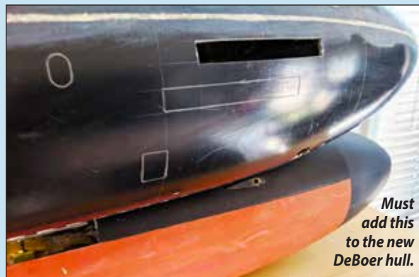
Fig. 11: Original SSY bow with scribing and Tube #1 opened up.
