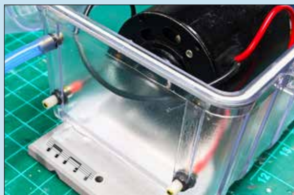
Fig. 26: External area where 2mm bullet connectors mate.
