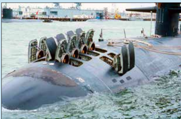
Fig. 13: Real Key West's open VLS hatches. Must add to new hull.
