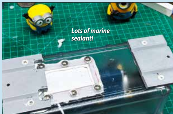
Fig. 22: Ventral view: Thermal window of Al plate; rail mounts.
