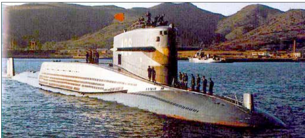
Fig. 20. Another photo of a Xia heading out to sea. Note the many limber holes in its missile turtleback.
