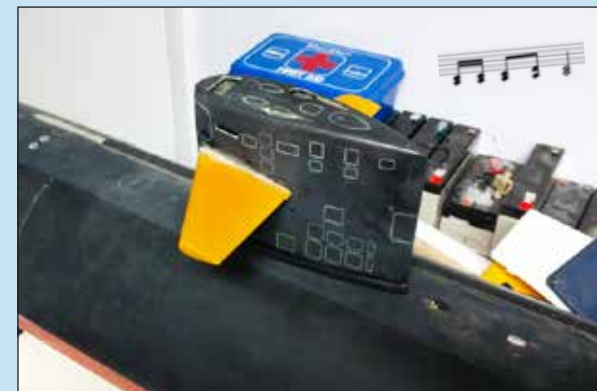
Fig. 3: Fitting the SSY sail with fairwater planes.
